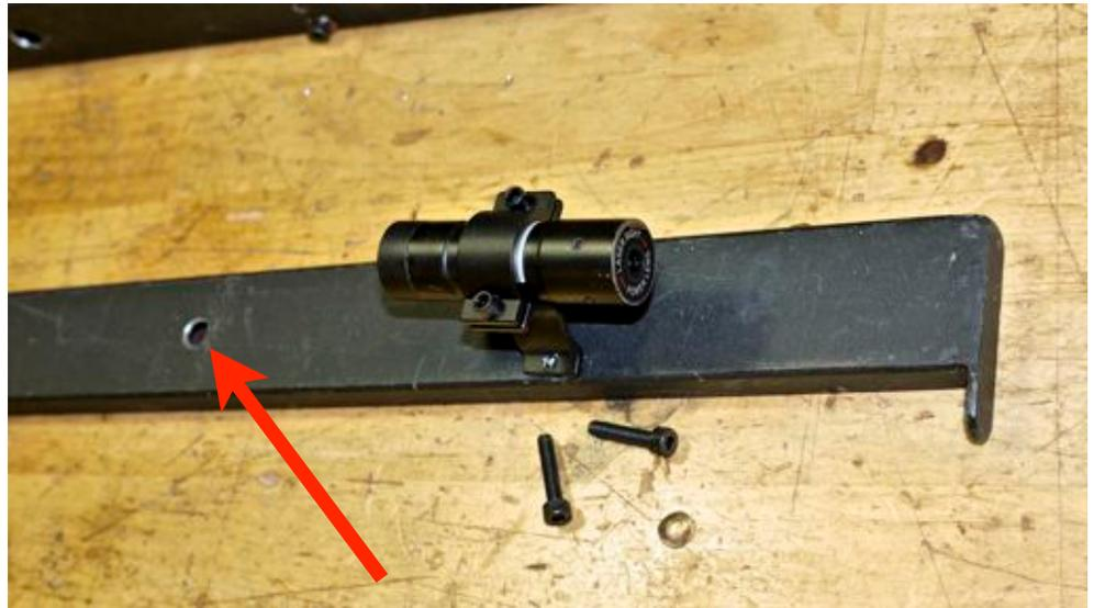
Use the short 4mm screws to attach the laser to the mounting base. Just snug
