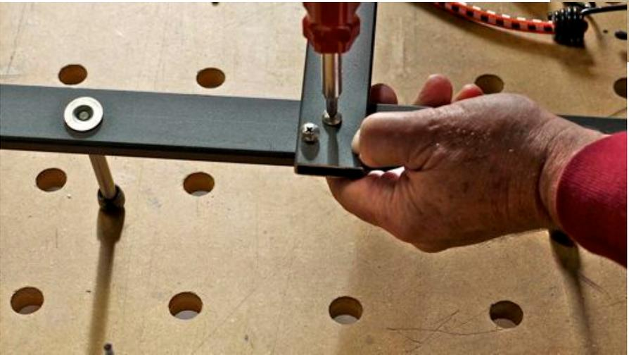
Now fasten the upper arm to the vertical member using a barrel nut and SS screw WITHOUT any adhesive. You want the upper arm to be able to rotate to fit properly on
