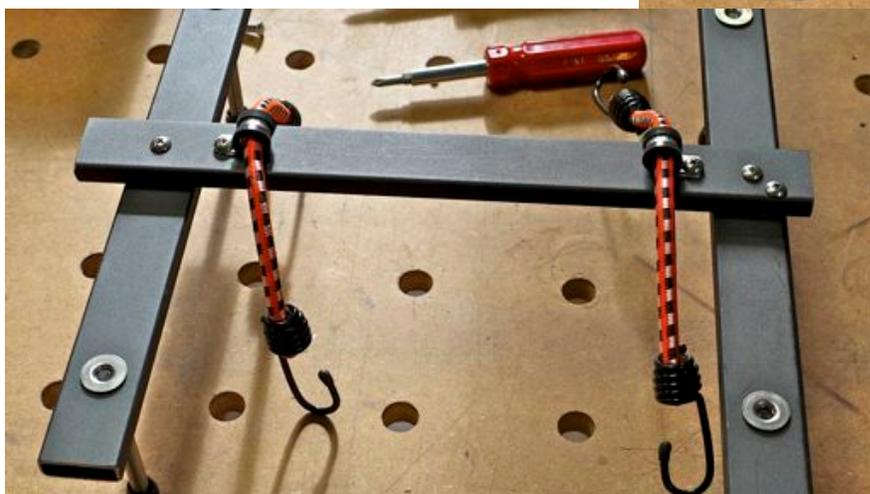
The final step is to screw the bungee cords to the vertical members with SS 10 x 24 screws and the padded clamps. This will keep the bungee cords from getting lost over time.
