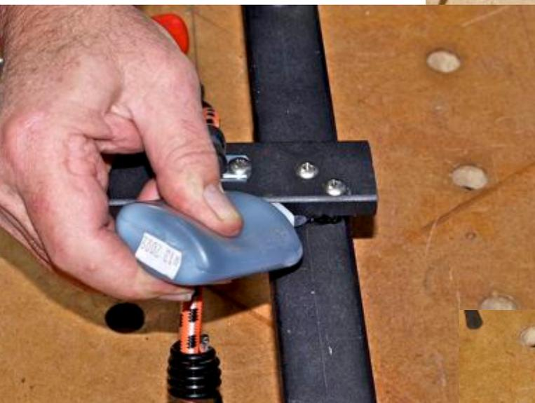
epoxy to reinforce the lower arm to vertical member joint. I also suggest adding a bit of CA or epoxy to keep the stand off pins or the weld nuts from loosening.
