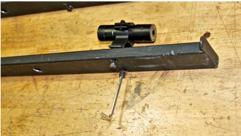
The next step is to adjust the laser beam to be as close to parallel with the arm as you can get it. Place the arm with the laser mounted onto a long level surface like the Stabila level shown here. Measure the height of the laser beam up close to the laser and as far away as you can.
